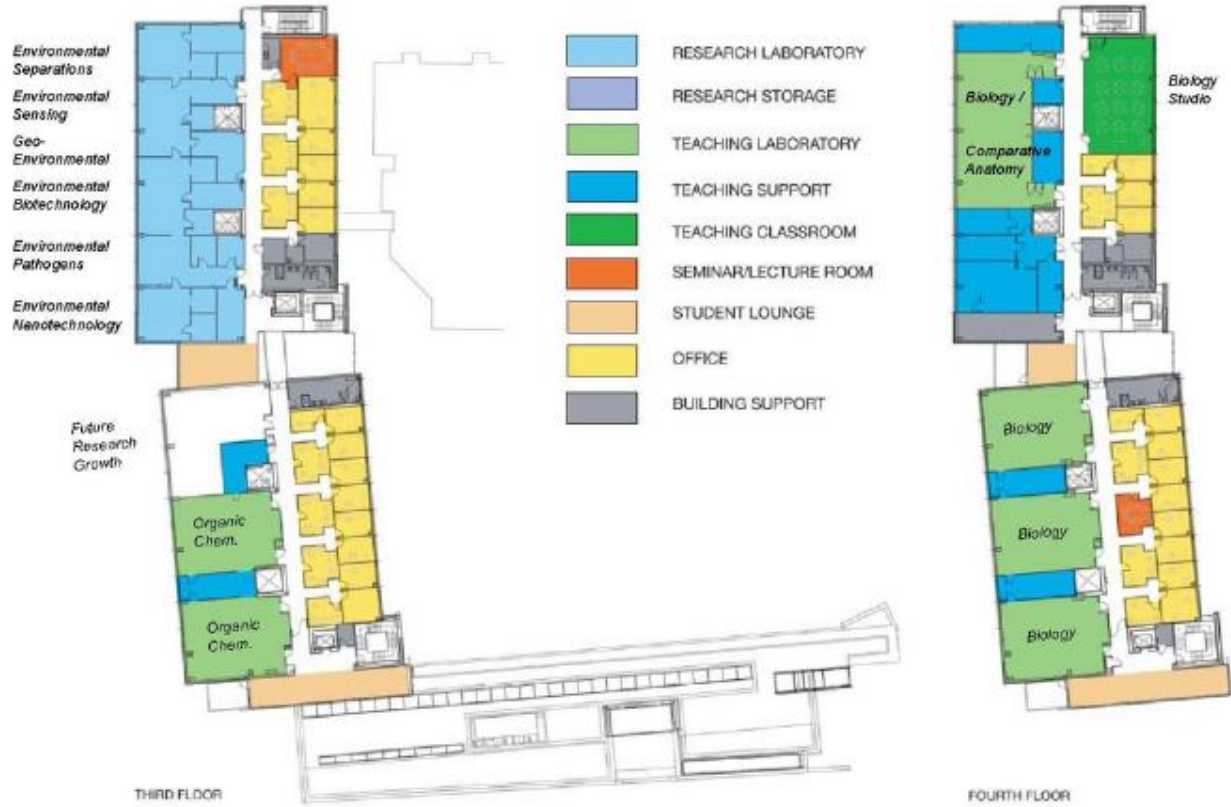
Figure 13: Typical Architectural Floor Plans
